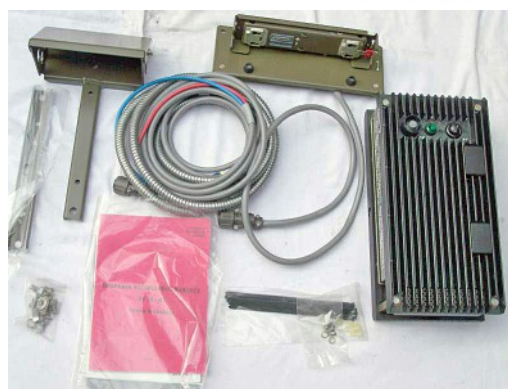
Vehicle charger kit N1 was designed for quick charge of RF-10 batteries in the field under combat conditions.
