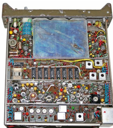
Internal view of RF-10. The cast aluminium alloy front panel had a frame to protect the controls from damage. The set had 11 different boards, interconnected by thin wires with Teflon insulation.
