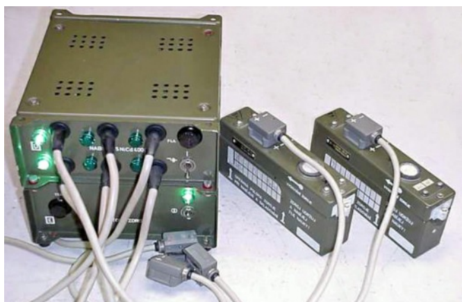
The standard desktop charger for 6 batteries was composed of the E + D box. This combination was AC mains powered. In emergency a battery could also be charged via the vehicle A box.
