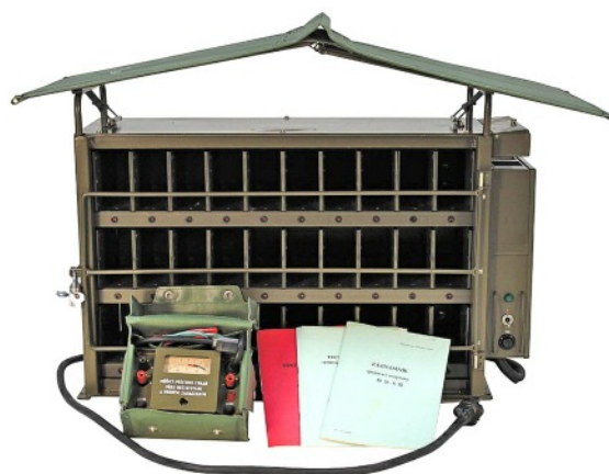
Conservation unit K-30 was used for long-time storage of up to 30 batteries.
