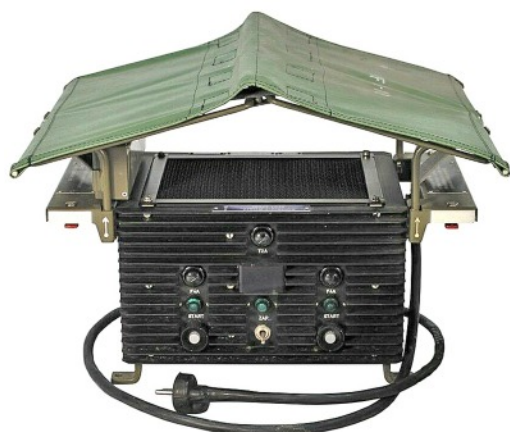
Quick charger N2 could charge 2 RF-10 batteries simultaneously in 1 hour. Both N1 and N2 chargers were not allowed to be used for normal operation, as it does not monitor the battery status but only the charging current for 1 hour. Imperfectly discharged batteries would overcharge and destroy their life span. It was developed for combat deployment only.
